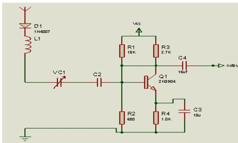
Figure 5: Schematic diagram of the LC tuning circuit.
