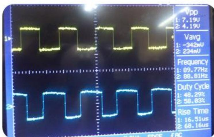
**Plate 1(c):** Input digital signal compared to the demodulator output digital signal after signal conditioning as tapped from the comparator inverting terminal.
