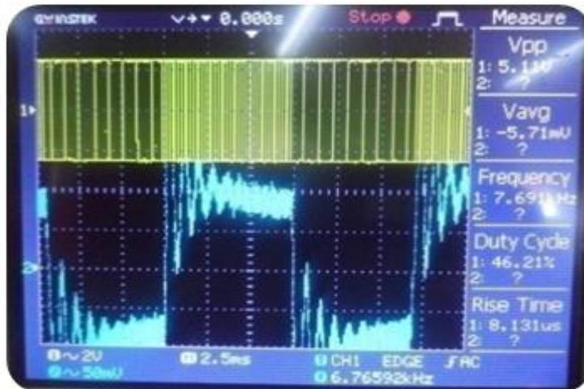
Plate 1 (a): Obtained FSK signal at a frequency of 4 KHz for the low bit and 8KHz for the high bit compared to the demodulated digital signal before filtering.
