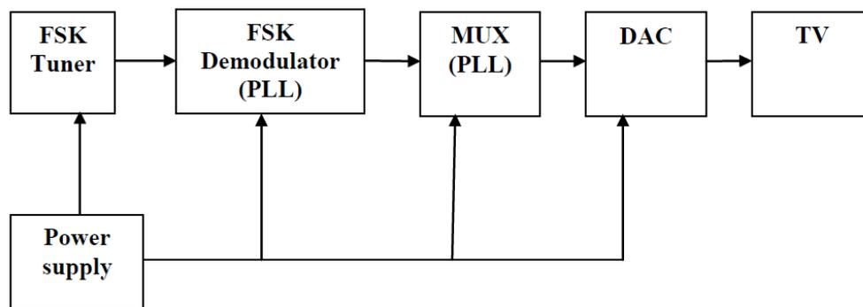
Figure 1: Block diagram of decoder.
