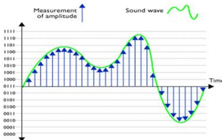
Figure2: Digital level sampling by a DAC.
