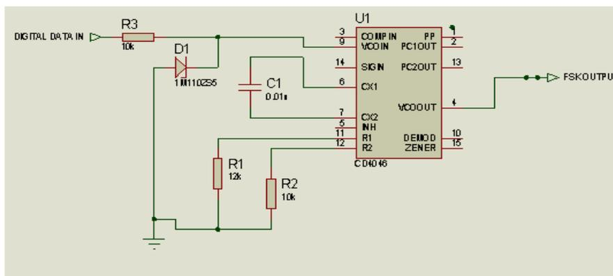
**Figure 4:** Schematic diagram of the FSK modulation circuit.
