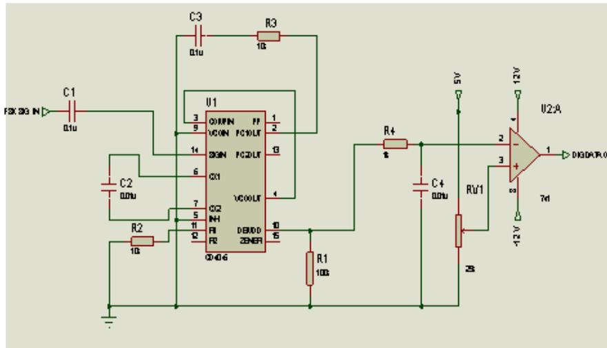
**Figure3:** Schematic diagram of the FSK demodulation circuit.
